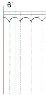
Figure 7: Cut 6" wide down entire length of panel
