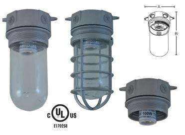
UL Listing: Suitable for wet locations for use in dwellings. Suitable for use with 90° C supply wiring. Complies with UL Standard 1598. For non-hazardous locations where the lamp, socket and wiring require protection from rain, corrosive fumes, non-explosive vapors and gases. Approved for maximum 100W incandescent.
