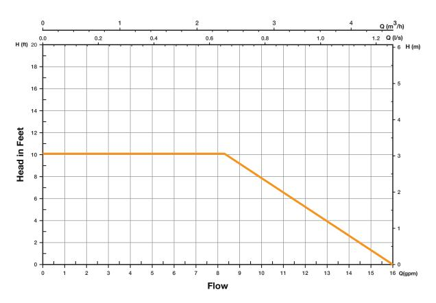
The 007e performance is ideal for hydronic zoning to reduce velocity noise or banging of zone valves closing against high head pressure circulators.
