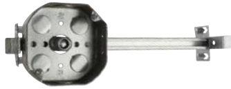
54151 J 1/2 Mounted on 6010-DW bar adjustable 10 1/2" to 18 1/2". Offset for 1/2", 3/4" or 7/8" plaster. Maximum horizontal positioning. 3/8" fixture stud.
