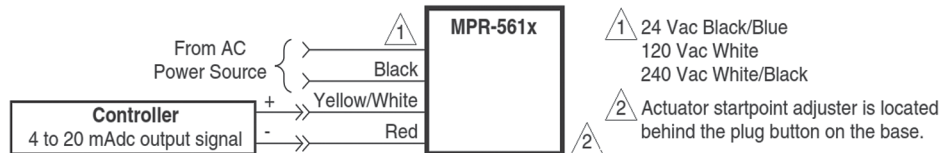
Wiring Diagram 4...20 mAdc Controllers
