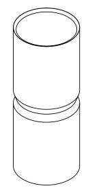
Unless otherwise specified, All overall length, height and socket bottom to socket bottom dimensions are to be  $\pm$ 1.1/2". All fitting angles are to be  $\pm$ 1.1 degree.
