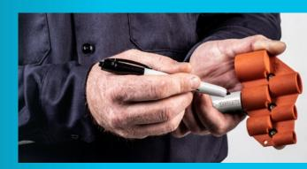
Step 3 Mark the pipe using the depth gauge tool
