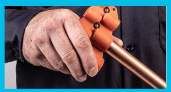
Step 2 Deburr the end of the pipe to remove any sharp edges.
