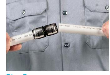
Step 2 **Examine the EvoPEX fitting and** SharkBite PEX tubing
