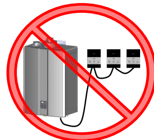
Controllers wired in series
