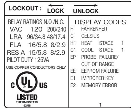
Figure 4: Lockout Switch
