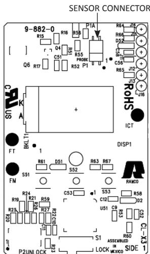
Figure 9: Sensor replacement on Display (Upper) Circuit Board.
