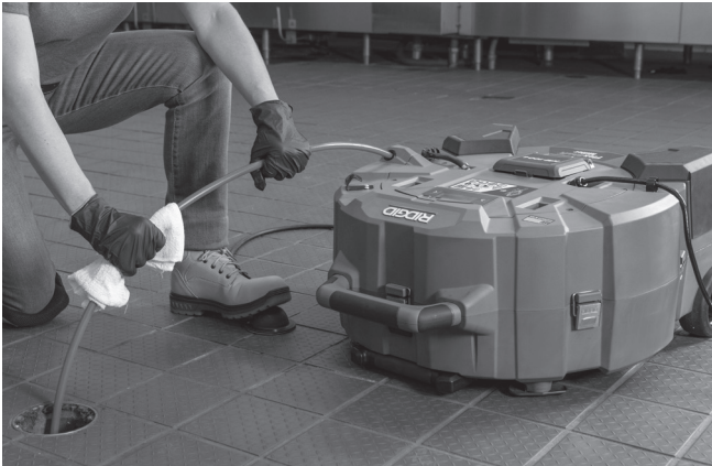
Figure 15 – Wiping Cable Off While Retrieving
