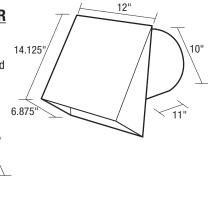
Fits 8" round duct Backdraft damper 22 gauge, galvanized steel construction
