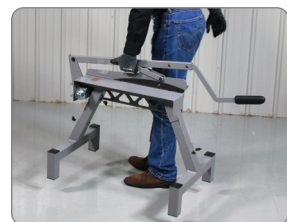
After securing the blade lock-pin in place, the SRCSC1 stone coated roofing cutter is safe to carry on to the job site.
