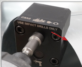
Begin crimping at angle
