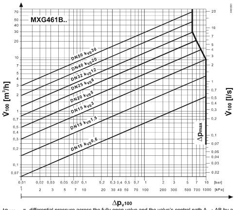
$\Delta p_{V100}$  = differential pressure across the fully open valve and the valve's control path A  $\rightarrow$  AB by a volume flow  $\mathring{V}_{100}$
