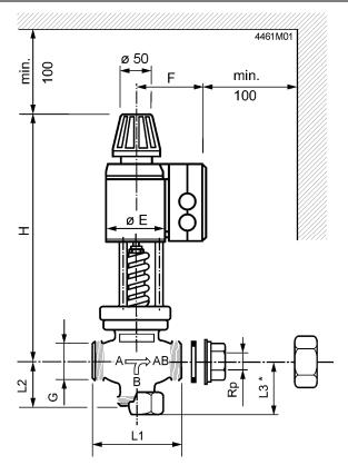
Externally threaded G...B to ISO 228-1 Internally threaded Rp... to ISO 7-1
