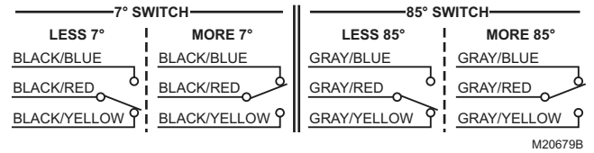
Fig. 6. Auxiliary switch wiring (S20 Series).
