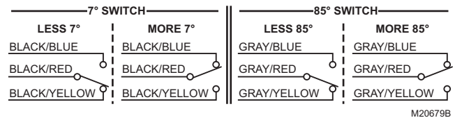
Fig. 11. SPDT auxiliary switch operation.
