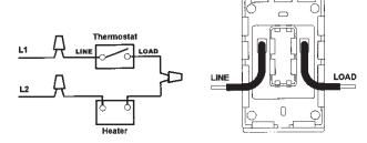
**CAUTION:** Do not short the 120 / 240 Vac wires with the thermostat. This will damage the thermostat and void the warranty.
