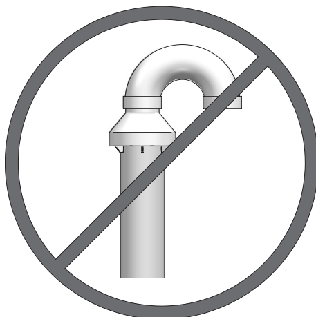
Figure 4-5 Do Not Install U-Bent to Rain Cap
