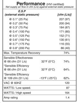
\*Sensible Efficiency - thermal \*\*Latent Efficiency - moisture Note: Effectiveness - based on temp, differential between the 2 airstreams Efficiency - takes into account all power inputs
