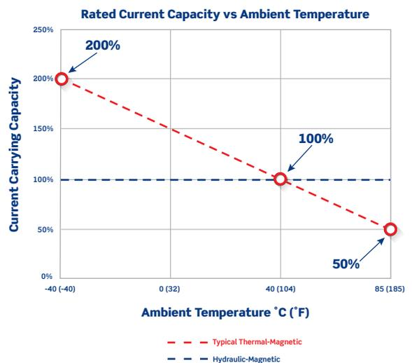
**Hydraulic-Magnetic trip technology helps prevent false tripping, even in extreme temperature ranges<sup>1</sup>, unlike traditional Thermal-Magnetic circuit breakers**
