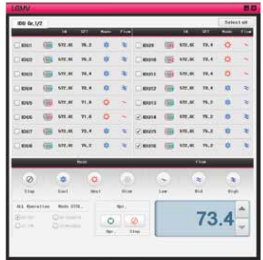
Figure 68: MV Control Indoor Units Screen
