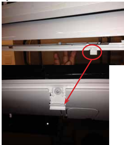
Figure 58: Remove Screws from Bottom Panel
