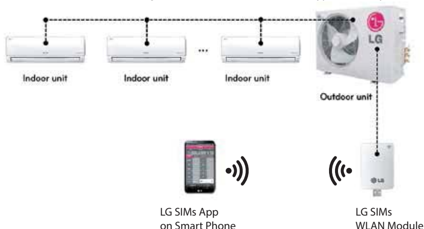
Figure 102: SIMS WLAN Module to Typical DFS System
