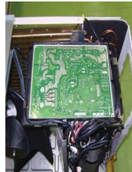
Tighten PCB Screws (6ea)
