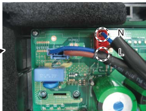
< Main PCB wiring Check Point >
