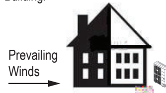
Figure 29: Leeward Side of the Building.
