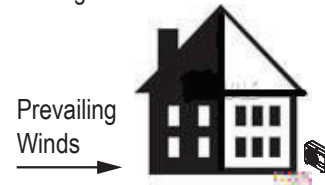
Figure 30: Leeward Side of the Building.
