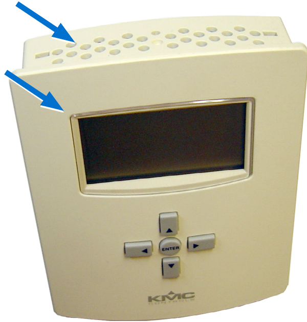
Clean Case Holes and Surface
