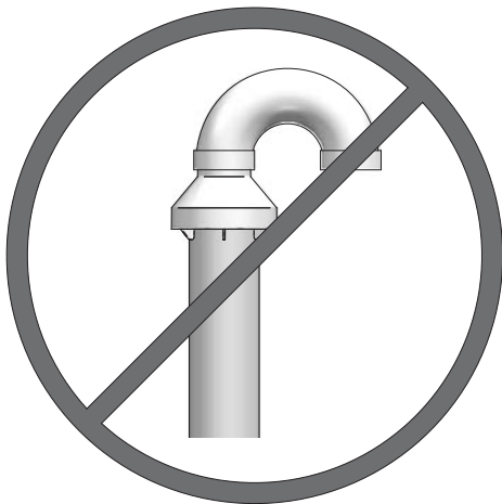
Figure 5-5 Do Not Install U-Bend to Rain Cap
