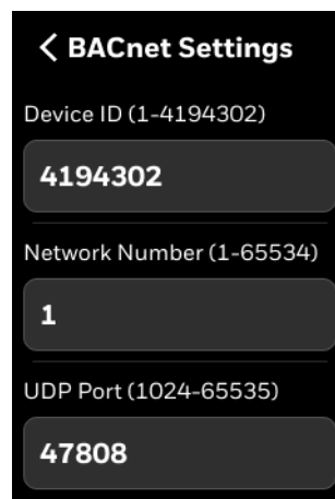
Figure 119 BACnet IP network settings
