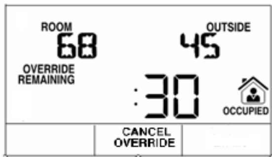
Fig. 42. Override display for Tenant.
