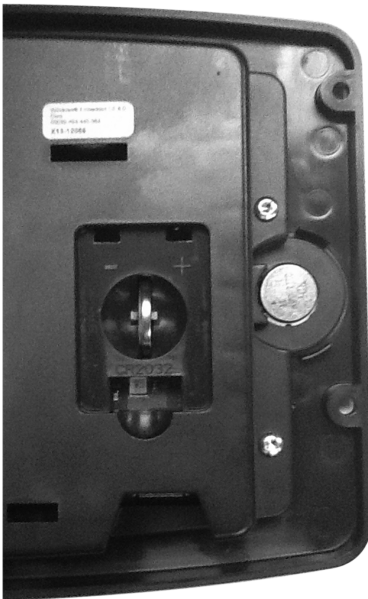
Fig. 5. Install CR2032 coin battery.
