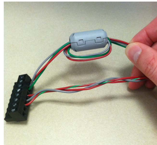
Fig. 3. Clamp filter in place.
