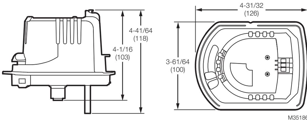
Fig. 1. Motor and damper dimensions in in. (mm).
