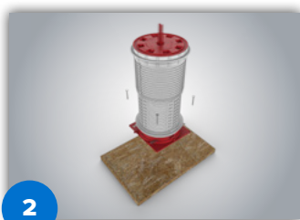
2 Secure sleeve to form deck, with cap installed
