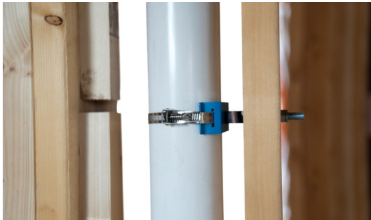
Vertical pipes or spiral ducts can be secured using a UNC1 Clip Kit and adding a 3/8" threaded rod that is bolted to the stud.
