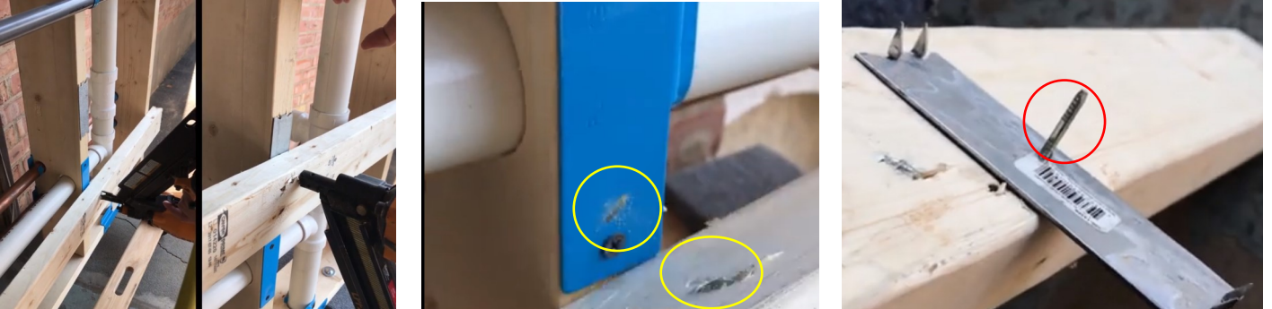
Firing with 100 PSI of pressure, the HAP Stud Guard deflects the nail while a common stud guard fails
