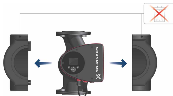
Fig. 3 Fitting insulating shells to the pump
