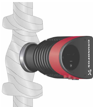
Fig. 13 Insulation of pump housing and pipework
