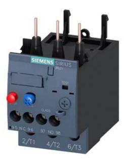
OVERLOAD RELAY 14...20 A FOR MOTOR PROTECTION SZ S0, CLASS 10, F. MOUNTING ONTO CONTACTOR MAIN CIRCUIT: SCREW TERMINAL AUX. CIRCUIT: SCREW TERMINAL MANUAL-**AUTOMATIC-RESET**
