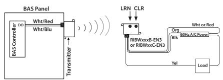
In this application the BAS system dry-contact output controls the transmitter and a RIBWxxxB-EN3 or RIBWxxC-EN3 is the receiver.
