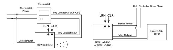
In this application the thermostat dry-contact output controls the transmitter and a RIBWxxxB-EN3 or RIBWxxC-EN3 is the receiver.
