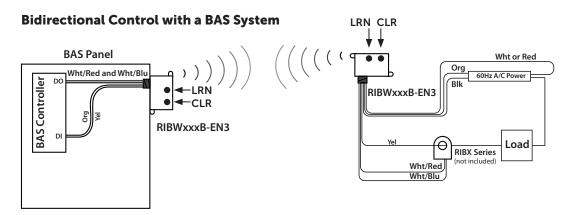
In this application the BAS system dry-contact output controls the transmitter on a RIBWxxxB-EN3. A second RIBWxxxB-EN3 receives the signal and activates it relay. A current switch detects current flow through the load and closes the dry-contact input on the second RIBWxxxB-EN3. The first RIBWxxxB-EN3 receives the transmission and closes its relay. This contact closure to the BAS system lets the controller know the load status.
