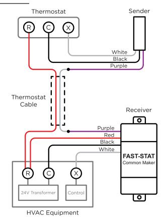
Generic Wiring Application (Dry-Contact Switching)
