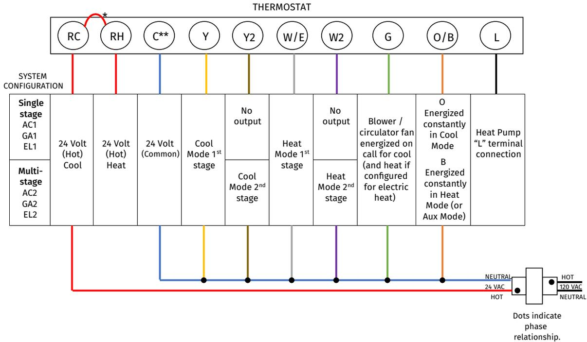
\*Internal jumper between RC and RH, located on back of thermostat above battery compartment.
