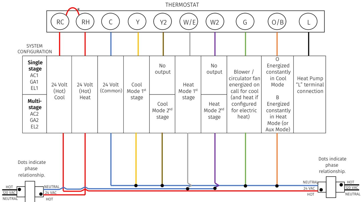
\*Two transformer systems (separate RC and RH wires), clip interna,RC/RH jumper located on back of thermostat above battery compartment.
