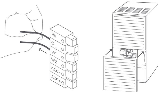
1. Check that all wires are properly inserted into the terminal blocks at the thermostat. Tug on the wires to ensure they are not loose.
