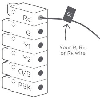
3. If you have only one R wire (either R, Rc, or R+), make sure it's inserted into the Rc terminal.
