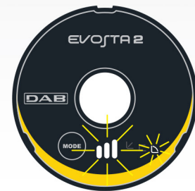
EVOSTA2 display with luminous segments indicating the type of set curve
