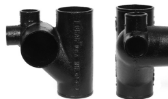
Part No. NH 458 Vented Closet Tee with 2" Top Vent and 2" Side Inlet (Left Hand or Right Hand; Designed for use below the floor; Fitting does not require a baffle.)
