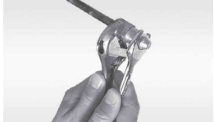
Figure 9 Carefully support the nozzle adapter when removing or installing nozzle
