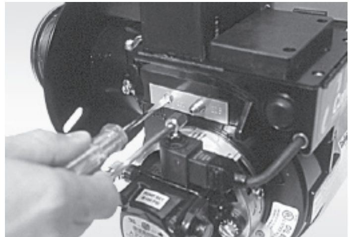
Figure 10 Installing head positioning bar
