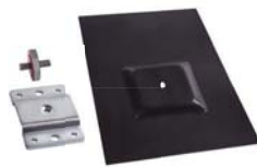
Flashing kit with 3/8" stud for attaching U mounts and other brackets using the supplied 3/8" stainless steel nut & washer. Black painted aluminum 6061 T6 flashing 14 3/4" L x 9 1/2" W x 0.6" H, galvanized steel base plate with six mounting holes and double stud.
