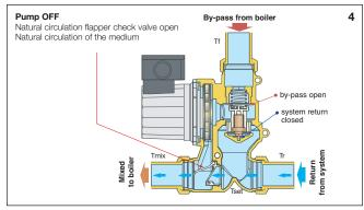
**Tf** = By-pass flow from boiler temperature, **Tset** = Boiler protection valve set point temperature, **Tmix** = Mixed water temperature, **Tr** = Return from system temperature
