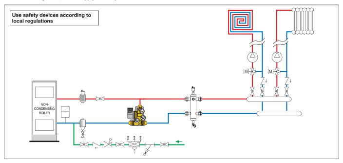
Non-condensing boiler, direct connection to buffer tank.
