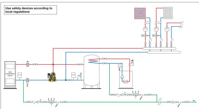
Non-condensing boiler, direct supply to the system.
