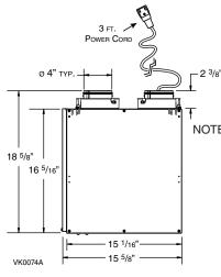
NOTE: ALL UNITS PORTS WERE CREATED TO BE CONNECTED TO DUCTS HAVING A MINIMUM OF 4" DIAMETER, BUT IF NEED BE, THEY CAN BE CONNECTED TO BIGGER SIZED DUCTS BY USING AN APPROPRIATE TRANSITION (E.G.: 4" DIAMETER TO 5" DIAMETER TRANSITION).
