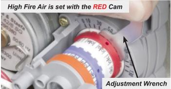
An old air setting specification of 7 is equal to 70° on the damper position scale of this new damper actuator.
