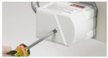
After you complete your adjustments make certain the disengaging pin has been reengaged with the damper position set between the high fire and low fire limits. Replace the actuator cover, making sure it is correctly seated, and test the burner for proper firing at low fire, high fire and in transition between low and high
