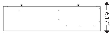
UVC Ceiling Fixture Side View
