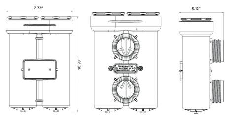
**Note** The stand-alone filter can be fitted to 1-5/8" pipework providing the end of the pipe is threaded with a  $1\frac{1}{2}$ " NPT tapered thread. For all other pipework types and sizes, adapters will need to be used.
