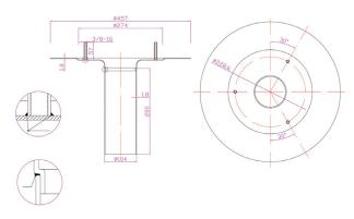
4" Aluminum New Construction Flat Deck Drain
